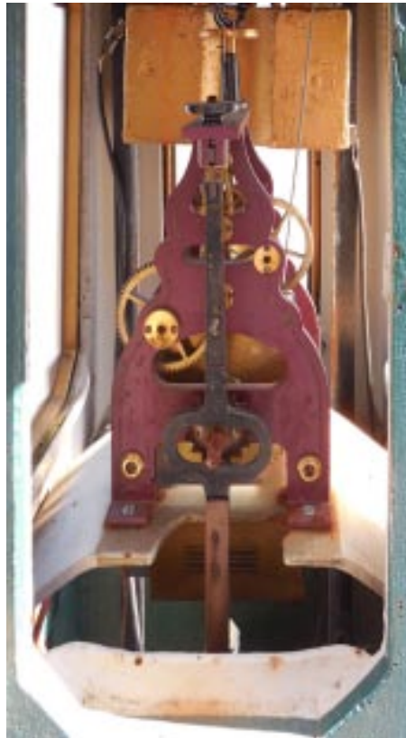
Above: As seen through a window at its base, the "Howard" movement at the heart of Mayer's clock.
